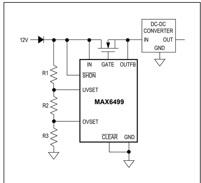
Figure 9. Overvoltage and Undervoltage Window Detector (MAX6499)
