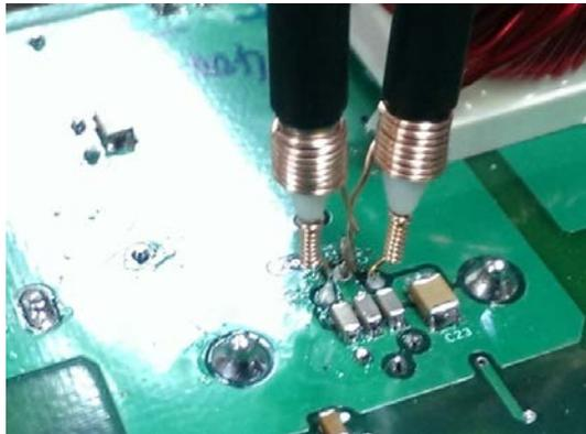
Figure 10. Low-inductance probing of fast, high-voltage signals
