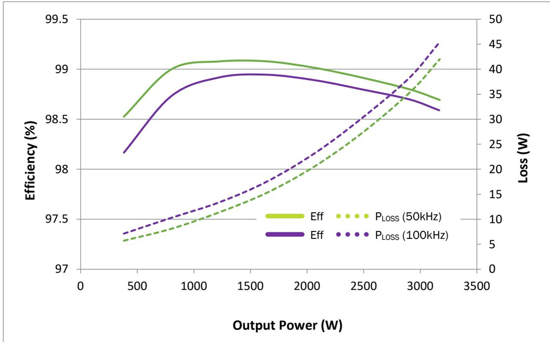
**Figure 6. Typical efficiency: 420V<sub>DC</sub> input, 240V<sub>AC</sub> output**
