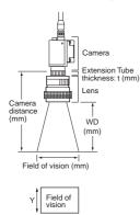
Note: 1. The lengths of the fields of vision given in the optical charts are the lengths of the Y axis.2. The vertical axis represents WD for small cameras.
