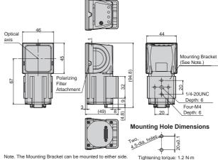
Tightening torque: 1.2 N·m
