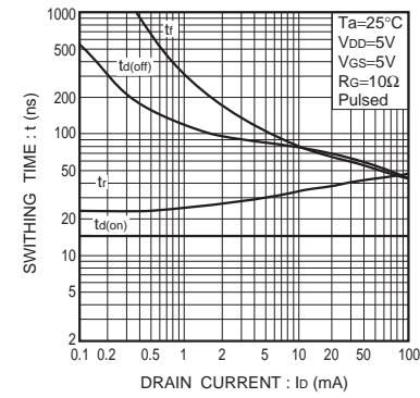
Fig.14 Switching characteristics
