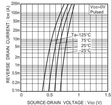
Fig.11 Reverse drain current vs. source-drain voltage ( I )
