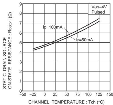
Fig.9 Static drain-source on-state resistance vs. channel temperature
