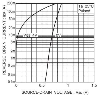
Fig.12 Reverse drain current vs. source-drain voltage ( II )
