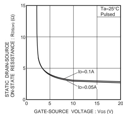
Fig.8 Static drain-source on-state resistance vs. gate-source voltage
