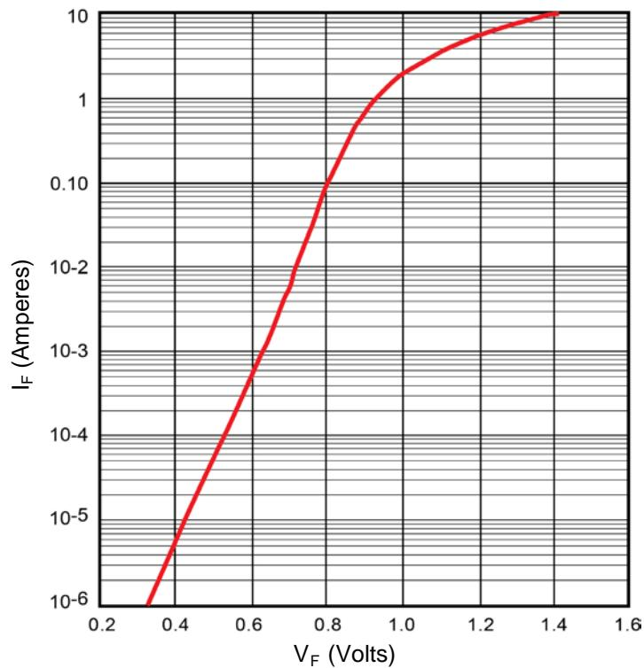
**FIGURE 4 – FORWARD CURRENT vs FORWARD VOLTAGE (TYPICAL)**
