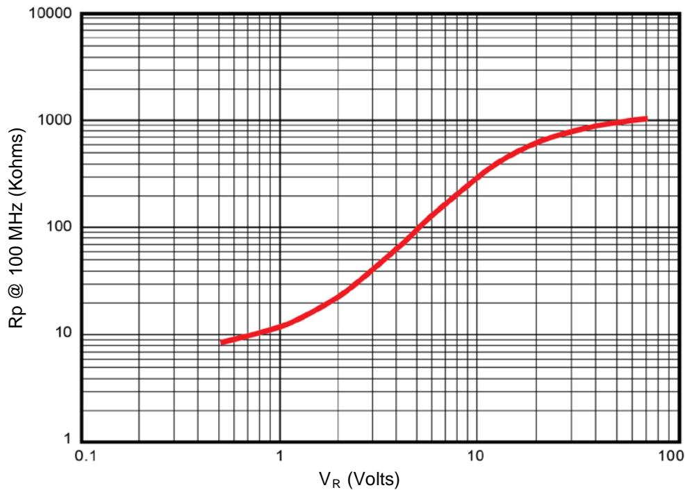
**FIGURE 3 – PARALLEL RESISTANCE (TYPICAL)**
