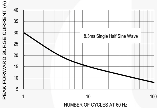
Figure 3. Maximum Non-Repetitive Forward Surge Current
