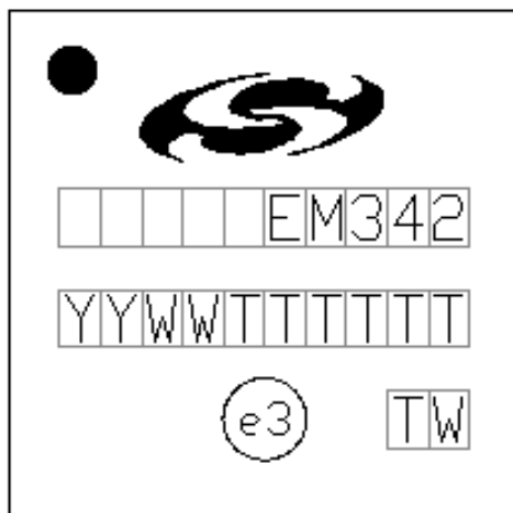
Figure 19.1. Part Marking for EM342
