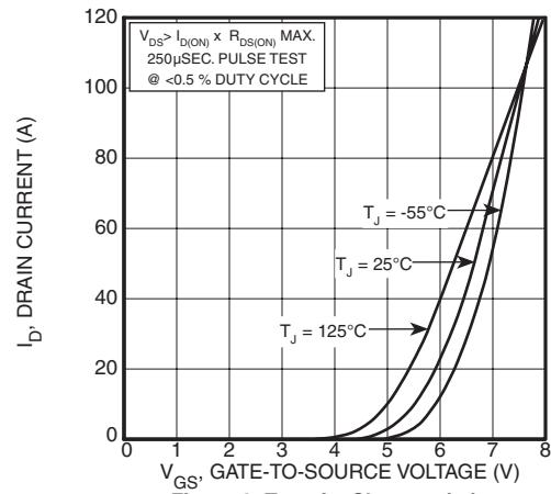
Figure 4, Transfer Characteristics
