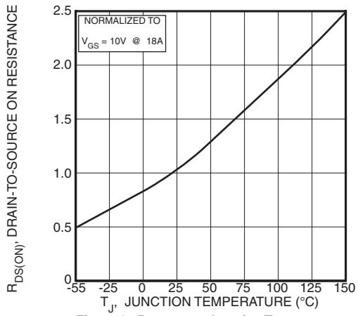
Figure 3,  $R_{DS(ON)}$  vs Junction Temperature
