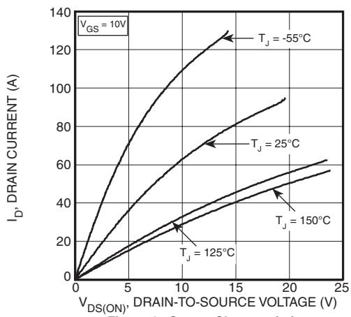
Figure 1, Output Characteristics
