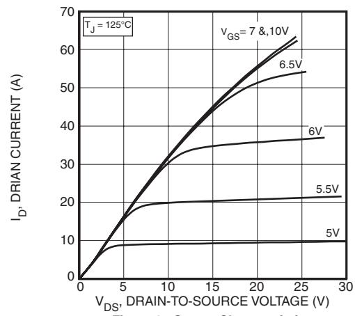
Figure 2, Output Characteristics
