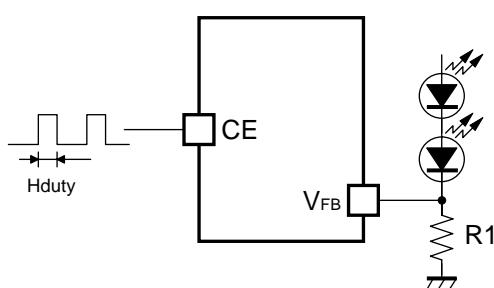
Dimming control by CE pin input
