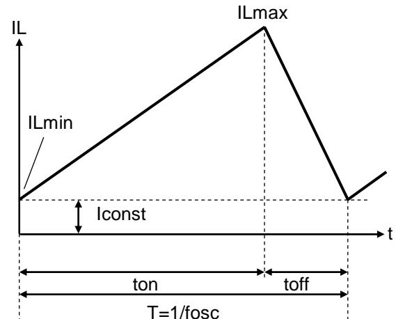
There are two operation modes of the step-up PWM control-DC/DC converter. That is the continuous mode and discontinuous mode by the continuousness inductor.
