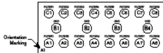
CM1442-08CS/CP 20 Bump CSP Package
