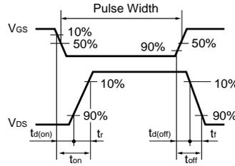
Fig.1-2 Switching Waveforms
