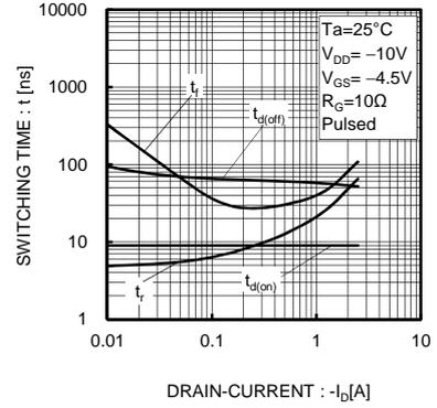
Fig.12 Switching Characteristics
