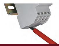
To remove the enclosure from the DIN rail, insert a screwdriver into the exposed slot in the tab and pull the tab down. Pull enclosure forward and remove from the rail.
