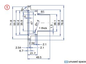
24 Terminal with 16 Standard and **8 High Current Terminals Horizontal PCB Screw Clamp**
