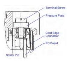
of K7075P, K70100P and K70150P and bug directly onto the board(s). **Solder Pins** are also provided in these enclosures for terminal-to-board connections when mounting an additional board directly behind the front cover. A **Wire Jumper** can be soldered to these pins as well.
