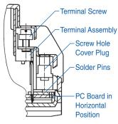
pressure plate ensure positive retention of the wires. The flat bottom of the terminal extends to the inside of the enclosure and provides the terminal-to-board connection. The terminal screws can be turned by a flat tip or a #2 Pozidriv screwdriver.
