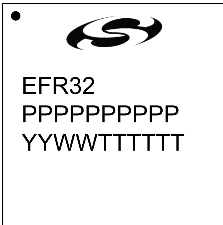
Figure 7.3. BGA125 Package Marking
