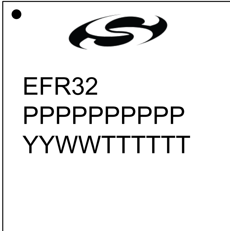
Figure 9.3. QFN68 Package Marking
