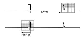
Figure 29. Trigger Delay or Pre-trigger View
