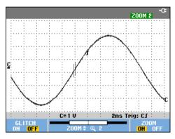
Figure 24. Zooming in a Waveform
