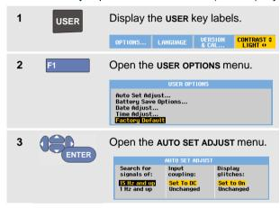
If the frequency range is set to > 15 Hz, the Connect-and-View function responds more quickly. The response is quicker because the test tool is instructed not to analyze low frequency signal components. However, when you measure frequencies lower than 15 Hz, the test tool must be instructed to analyze low frequency components for automatic triggering:
