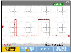
Figure 33. Triggering on Narrow Glitches
