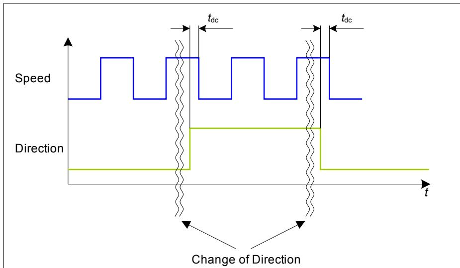
Figure 4 Timing Definition of the Direction Signal
