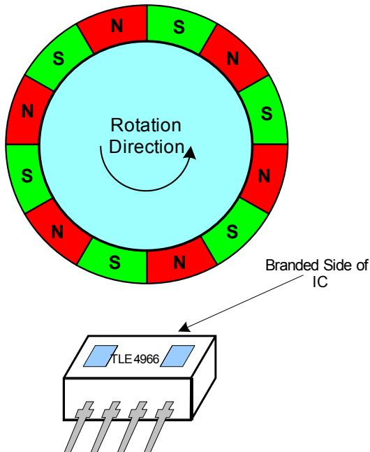
**Figure 5** Definition of the Direction Signal
