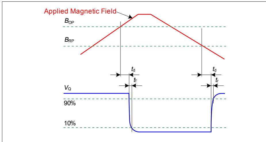
Figure 3 Timing Definition of the Speed Signal
