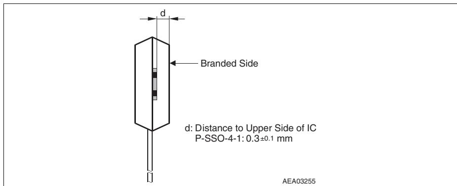
**Figure 8      Distance Chip to Upper Side of IC**
