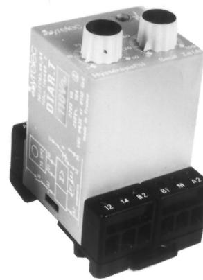
The DIAR.T is a current control which is capable of sensing up to 100 Amps. If requires a stepdown transformer, T1 100. The transformer has a 0.4" diameter center hole through which a current carrying lead is routed. Automatic or manual unlatching is available in each unit.
