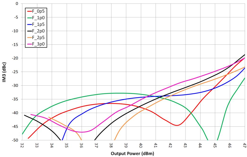
**Figure 6 - IM3 vs. Output Power of the CG2H30070F
