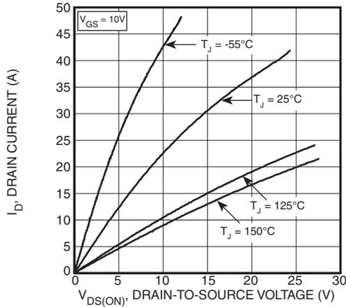
Figure 1, Output Characteristics
