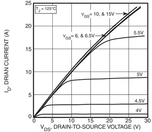
Figure 2, Output Characteristics
