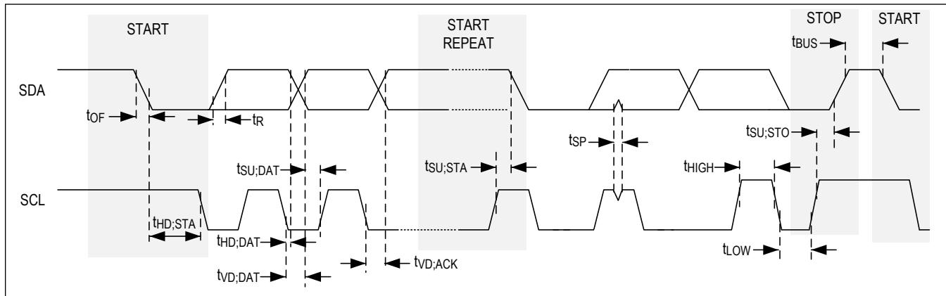
Figure 3. I<sup>2</sup>C Timing Diagram
