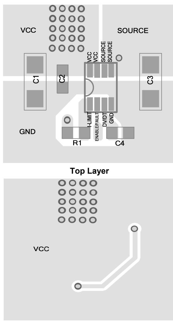
**Figure 3—Recommended PCB layout**
