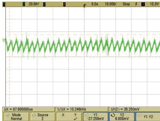
Figure 5. Output Noise,  $V_{IN}$  36V,  $I_O$  12A
