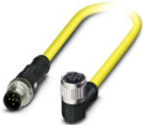
Sensor/Actuator cable, 5-position, Plug straight M12-SPEEDCON, A-coded, on Socket angled M12-SPEEDCON, A-coded, Cable length: 0.5 m
