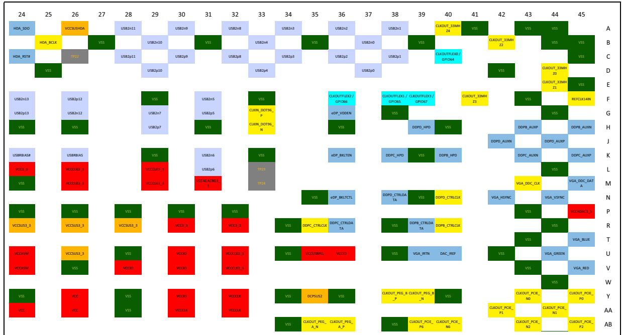
Figure 6-8. Mobile PCH Ballout (Top View - Lower Right)
