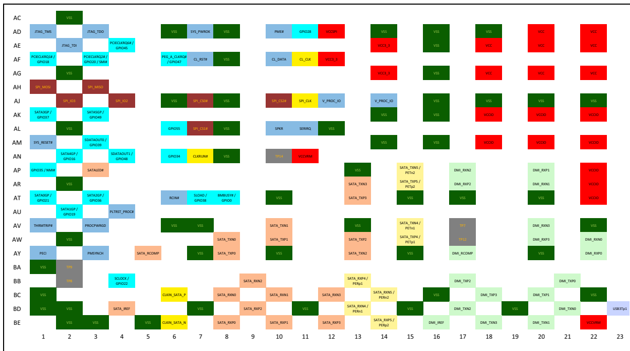
Figure 6-6. Mobile PCH Ballout (Top View - Lower Left)
