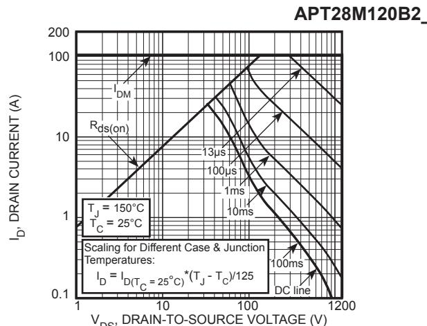
Figure 10, Maximum Forward Safe Operating Area
