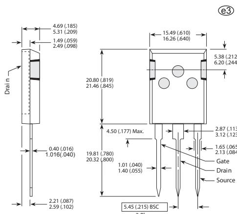
These dimensions are equal to the TO-247 without the mounting hole.
