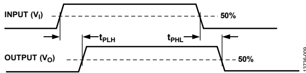
Figure 11. Propagation Delay Parameters
