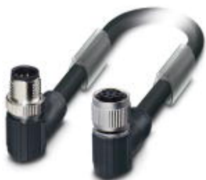
Bus system cable, VARAN, 6-position, PVC, black, shielded, Plug angled M12 SPEEDCON, A-coded, on Socket angled M12 SPEEDCON, A-coded, cable length: 15 m, Customer version
