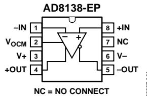
Figure 6. Pin Configuration
