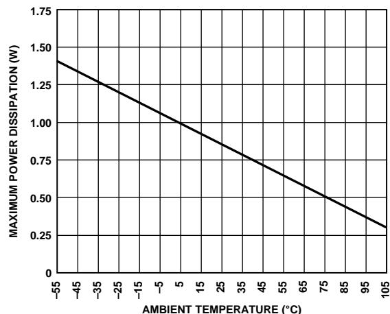
Figure 3. Maximum Power Dissipation vs. Ambient Temperature
